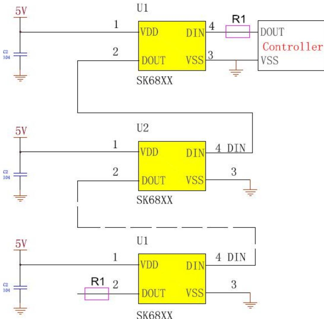
In the application circuit, the DIN signal is connected to the signal input and output terminals. In addition, in order to make the IC chip is more stable, even the capacitance between beads is essential back;
