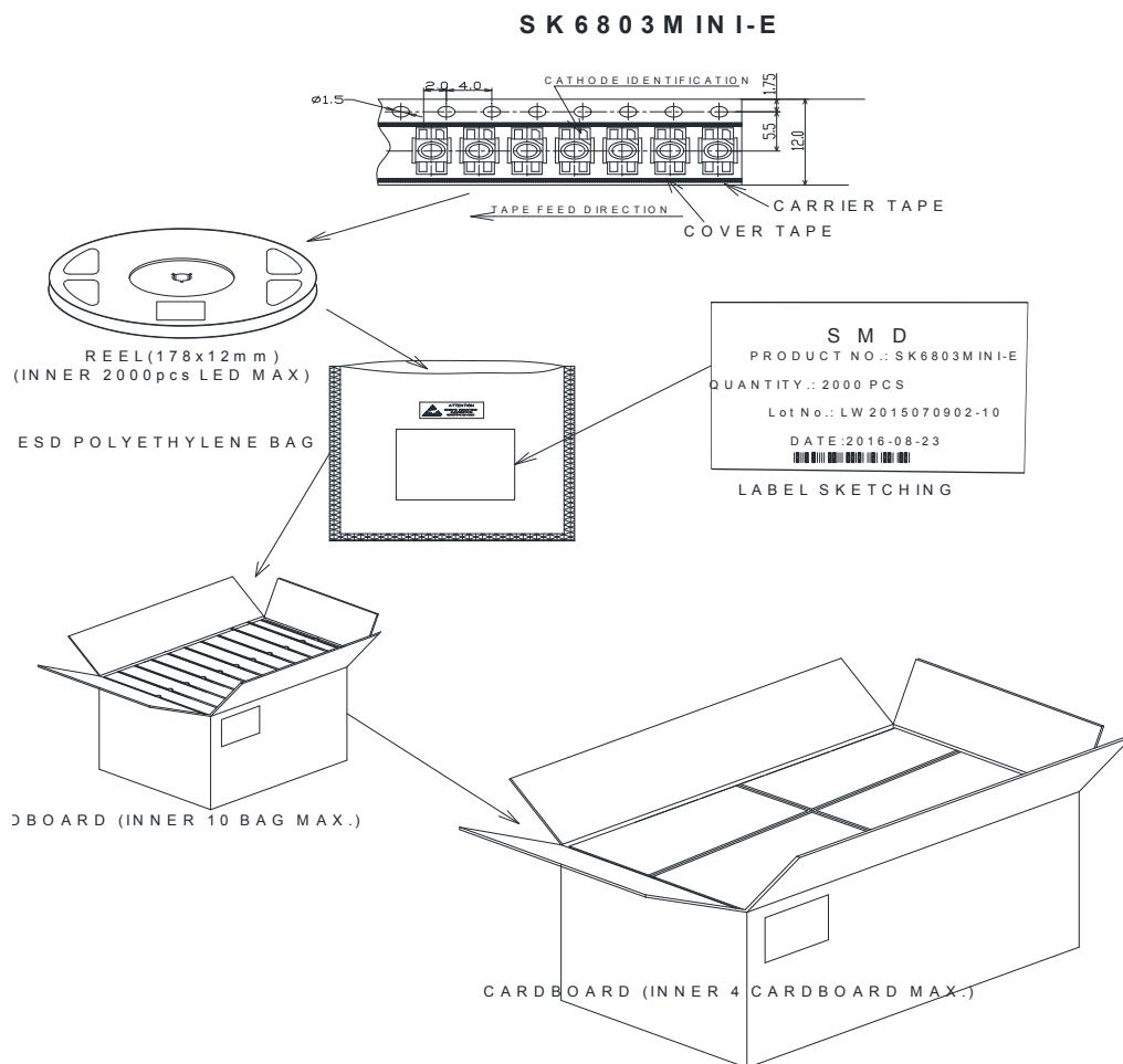
The reel pack is applied in SMD LED. The LEDs are packed in cardboard boxes after packaging in normal or anti-electrostatic bags. cardboard boxes will be used to protect the LEDs from mechanical shocks during transportation. The boxes are not water resistant and therefore must be kept away from water and moisture.
