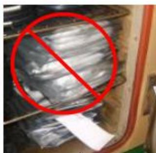
**Low-temperature dehumidifier must remove the bags, and then put tray in the oven**
