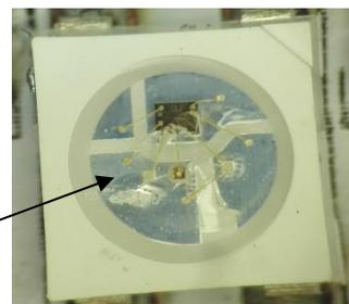
**1.1.1** This series of LED products use coating has moisture-proof anti-static aluminum foil bag, handling should be avoided in the process of extrusion, packing bags of pierced happens, at the same time to prepare the necessary electrostatic protective measures. Above line homework before LED packaging already exists leakage or damaged, please stop using directly, the performance test of photoelectric packaging products with high-temperature dehumidification action again after use.
