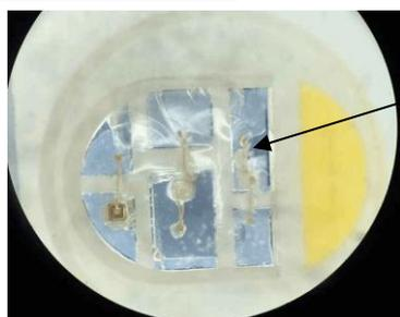
Plastic cracking caused by moisture infiltration and S5050RGBW rainbow phenomenon
